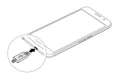
After fully charging, disconnect the device from the charger. First unplug the charger from the device, and then unplug it from the electric socket.
