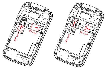
To remove the SIM card or microSD<sup>TM</sup> card, press down on the small plastic tab (1), then slide out the card (2). Do not use force or use any sharp objects.
